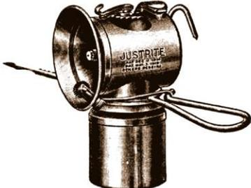
Lever wire valve feed. Adjustable candlestick and steel hook lighter attachment. 18 candle power. 2¾-inch reflector. Equipped with 23 jewel tip and No. 77 carbide can. Polished brass.
